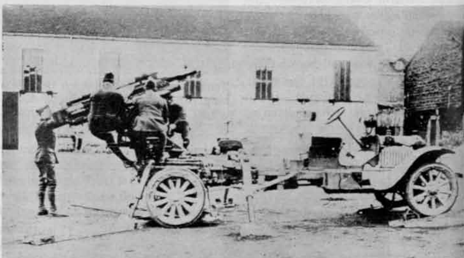
Figure 2—75mm AA truck mount
